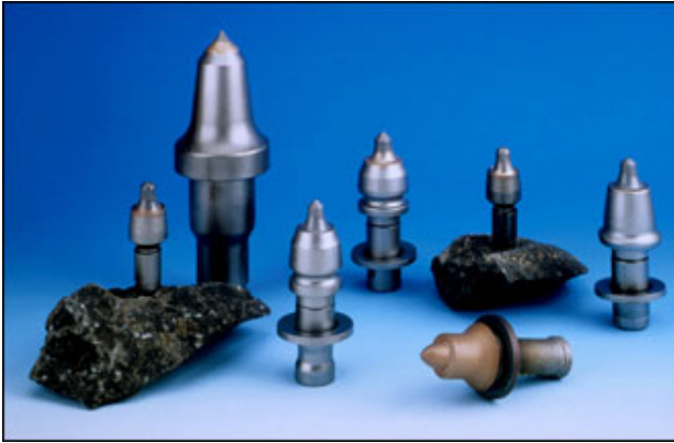
Photo 2: Mining chisel inductively brazed with brazing alloy BrazeTec 21/80 or 21/68, flux BrazeTec special h or h285. Brazing under an inert gas possible (N 2 /H 2 -mixture 95%/5%). Photo BrazeTec Hanau.
