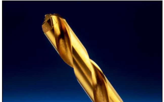
Photo 3: TiN coated drill inductively brazed with brazing alloy BrazeTec 6488 and flux BrazeTec special h. Photo BrazeTec Hanau.
