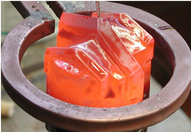
Photo 7: Induction brazing of a drill, Brazing Centre Hanau.
