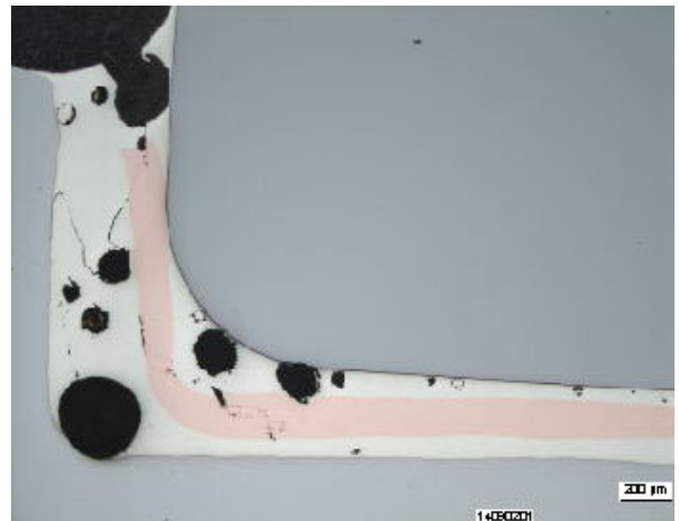
Photo 9: Porous brazed layer, too large a gap. Magnification 100:1. Photo Brazing Centre Hanau. The brazing alloy was overheated in the brazing process. The hard metal was inadequately secured.
