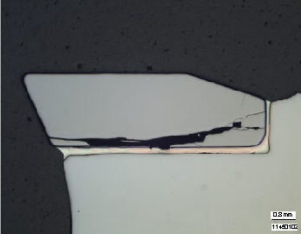
Photo 11: alloySaw tooth brazing with fracture lines in the hard metal. Magnification 12,5:1. Photo Brazing Centre Hanau. Overloading of the hard metal as a result of unfavourable forces or quality problems with the hard metal. Contour in the corner between the saw-body and hard metal not identical.
