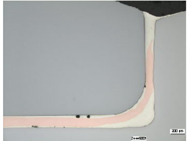
Photo 8: The brazing gap in a good brazed joint using tri-metal brazing alloy BrazeTec 49/Cu. Magnification 100:1. Photo Brazing Centre Hanau.
