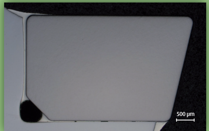
Figure 31 | Badly shaped saw blade body
